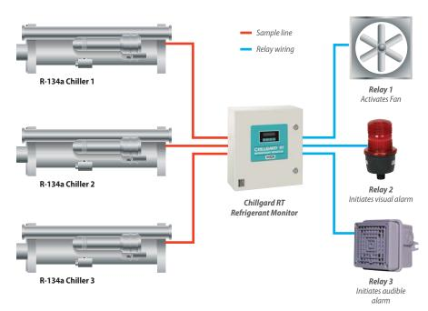
\*use of auxiliary relays may be required due to electrical load
